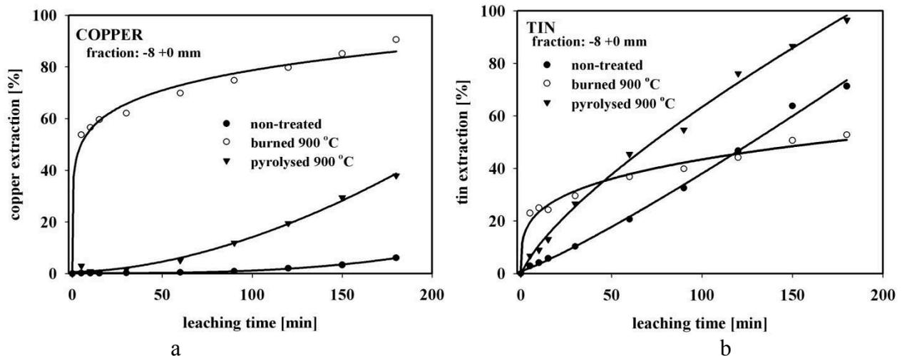
Figure 7 Leaching kinetic curves for (a) copper and (b) tin from untreated, burned and pyrolysed PCBs.
