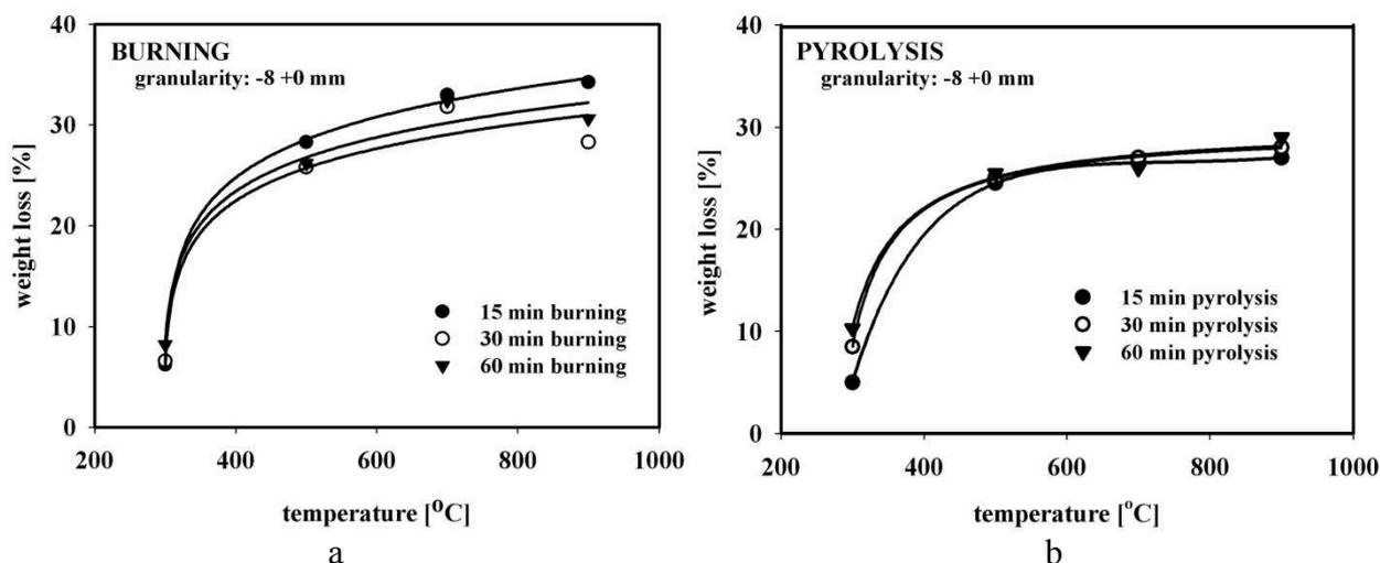
Figure 3 The temperature dependence of weight losses after (a) burning, (b) pyrolysis
