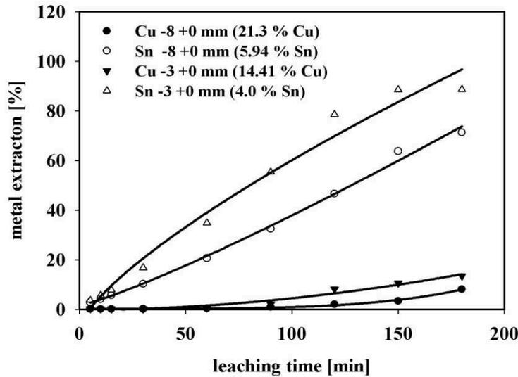
Figure 4 Kinetic curves of copper and tin leaching from non-thermal treated PCBs with various grain sizes
