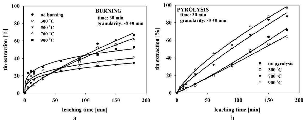
Figure 6 Kinetic curves of tin leaching from PCBs after (a) burning and (b) pyrolysis at various temperatures.
