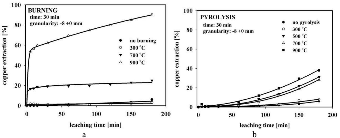
Figure 5 Kinetic curves of copper leaching from PCBs after (a) burning and (b) pyrolysis at various temperatures.
