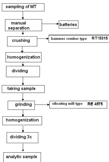
Fig. 2: The scheme of mobile phones sampling
