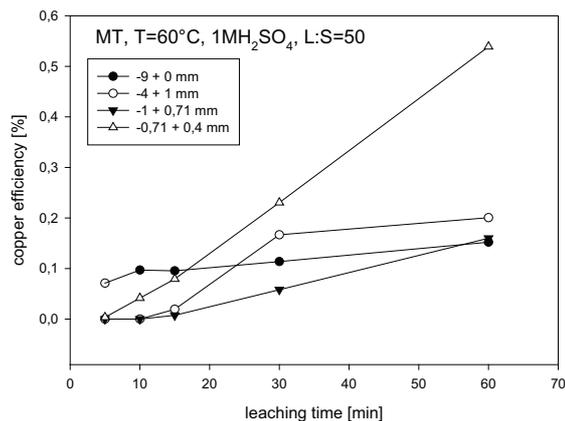
Fig. 7: The comparison of kinetic leaching curves of copper extraction on various fractions pre-treated MT
