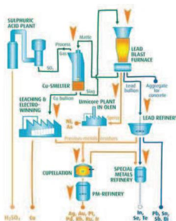
Fig.1 Flowsheet of Umicore's integrated smelter at Antwerp/Belgium [2]
