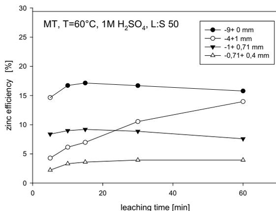
Fig. 6: The comparison of kinetic leaching curves of zinc extraction on various fractions pre-treated MT
