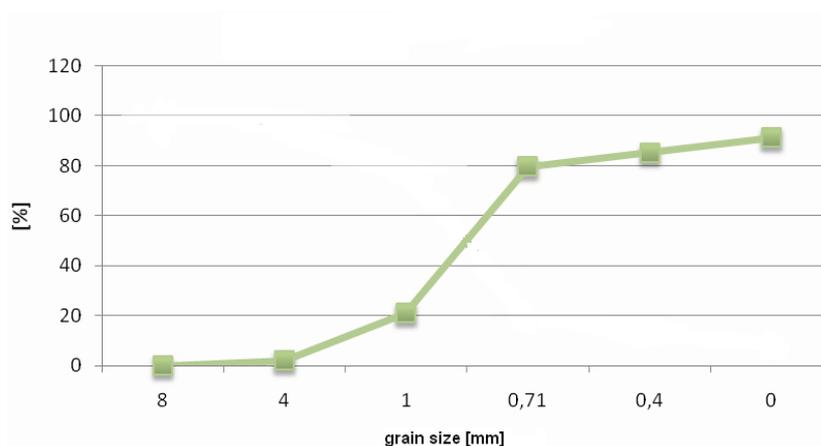
Fig. 3: Grading analysis of sample M1 (cumulative curve)
