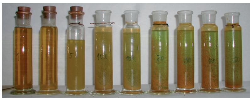
**Fig. 11: Hydrolytic precipitation of goethite from lixiviant**
